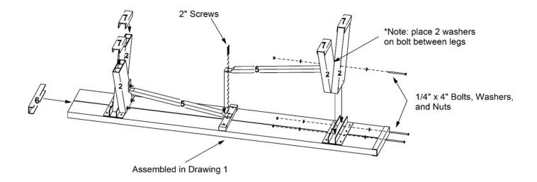
Insert one 15¾" leg (part 2) into bracket. Place second 15¾" leg (part 2) on inside of bracket and loosely fasten with 4" bolts, washers and nuts. Set 24¾" diagonal brace on inside of legs with ¼" drilled hole against legs. Using one 4" bolt, washers and nut, fasten diagonal brace to legs. When inserting bolt, place TWO washers in between legs. Tighten all bolts.
