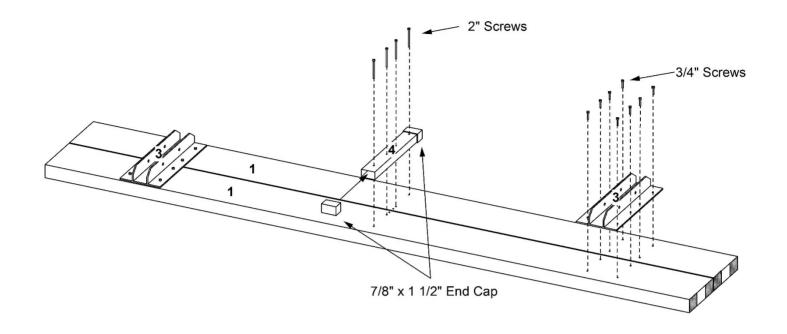
Lay out two 72" seat rails (part 1) with pilot holes facing up. Be sure wood inserts are flush with vinyl. Set two  $10\frac{3}{4}$ " seat brackets (part 3) over pilot holes at each end of seat rail, leaving  $\frac{1}{4}$ " gap between rails. Using eight  $\frac{3}{4}$ " screws per bracket, fasten each bracket to seat rails.
