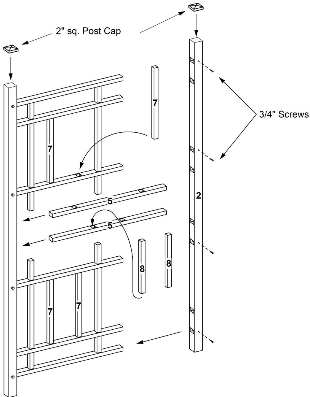
Insert two 27½" middle cross rails (part 5) into remaining routed holes in side of post, inserting free ends of 26½" vertical rails into middle cross rail. Insert four 16¾" vertical rails (part 7) into remaining holes in inside cross rails. Insert two 13" vertical rails (part 8) into remaining holes in middle cross rails. Insert free ends of cross rails into 74" right post (part 2).
