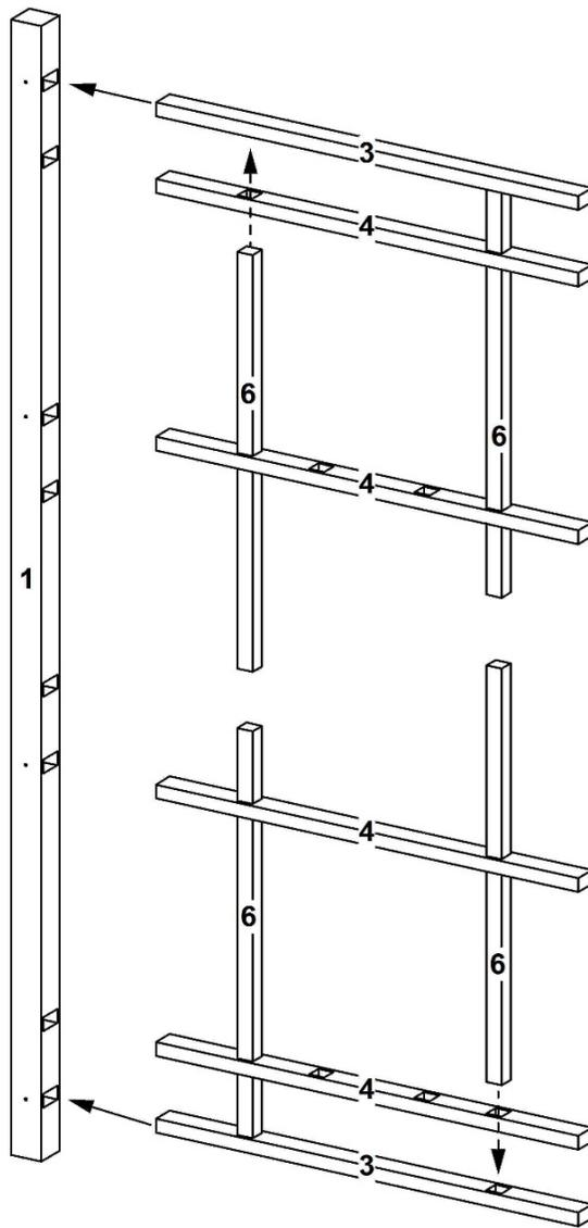
Starting at bottom of 74" left post (part 1), insert one 27½" outer cross rail (part 3) and two 27½" inner cross rails (part 4). When inserting two inner cross rails insert sides with four routed holes facing each other. Insert two 26½" vertical rails (part 6) through outer holes of inner cross rails and into outer holes of outer cross rail.
